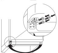
Move the door handle from the left to the right and cover the remaining holes with the hole cover pins attached.
